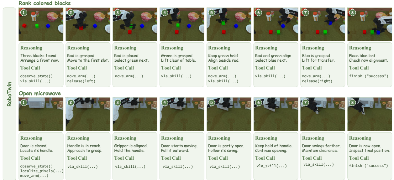
Figure 10 Examples of OmniBrain-0 on RoboTwin 2.0. Top: arranging colored blocks in a row. Bottom: opening a microwave.
